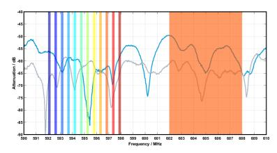
While narrowband microphones use individual 200 kHz links for transmission (left-hand side), WMAS technology uses employs time slots in a 6 or 8 MHz wide window (right-hand side). More information at sennheiser.com/wmas
